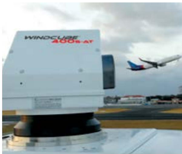
▲ LEOSPHERE wind shear monitoring equipment
